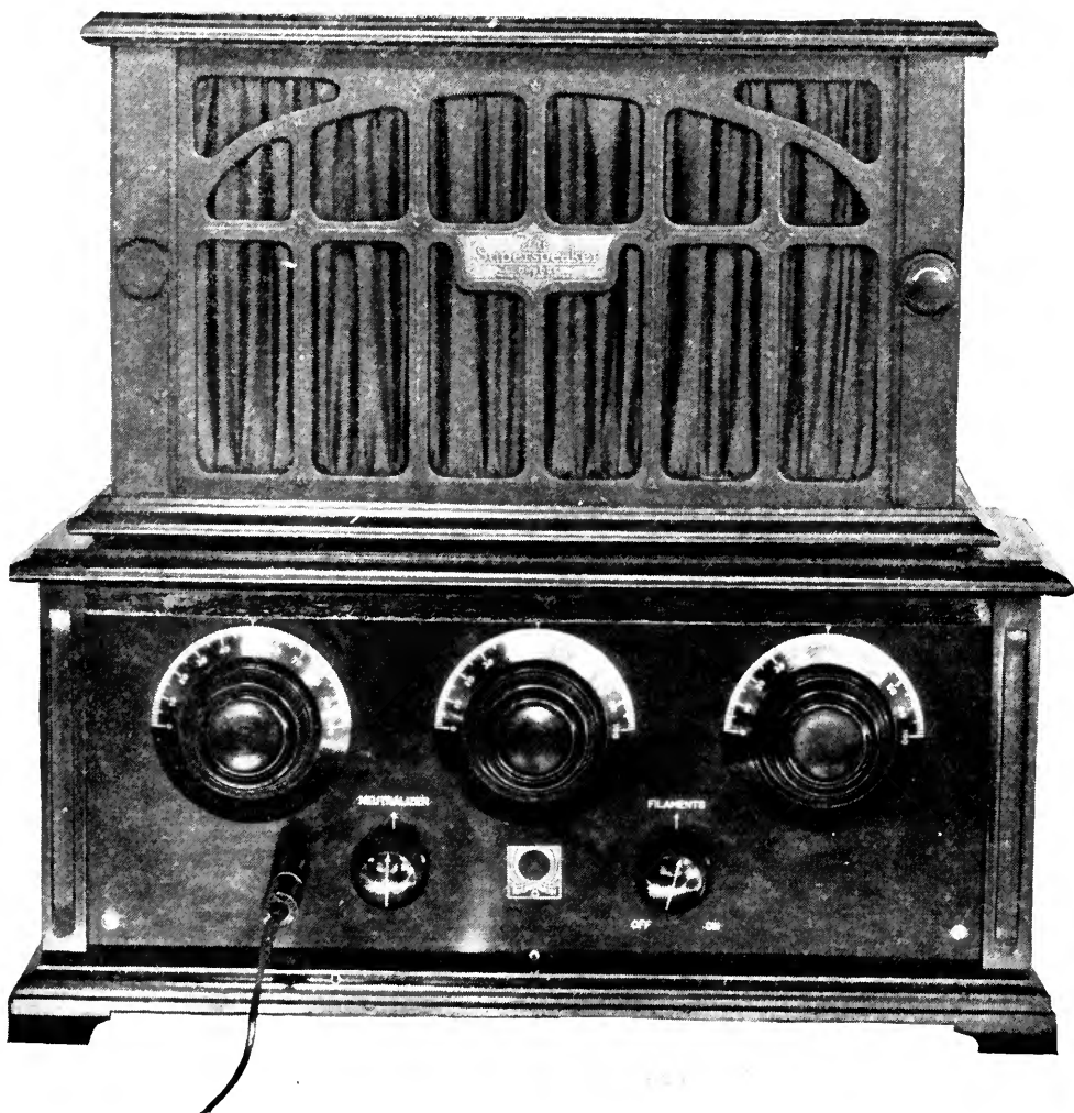
Two receivers and a loud speaker are illustrated in these photographs. The receivers are the Clearfield and the Richardson "5". They are both of the tuned radio frequency type. The Superspeaker Console speaker comes from the Jewett Radio and Phonograph Co.
